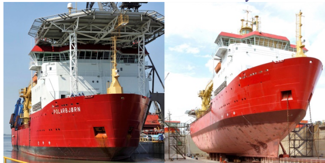
MV Polar Bjorn arrives for conversion in Odense shipyard, Denmark, May 2011. The most obvious external change was the relocation of the flight deck to the stern from its original position above the bridge.
